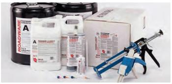
Roadware 10 Minute Concrete Mender™ is a high-penetration two-part hybrid urethane that WHEN combined with sand, forms a tough instant polymer concrete. This nearly water thin formula is designed to Microdowel™ deep into the host concrete creating extremely high bond strengths, reinforcement of the repair area as well as permanent repairs. Unlike epoxies or cementitious Grouts, Roadware 10 Minute Concrete Mender™ will not "pop-out" as it will not become brittle with time.
